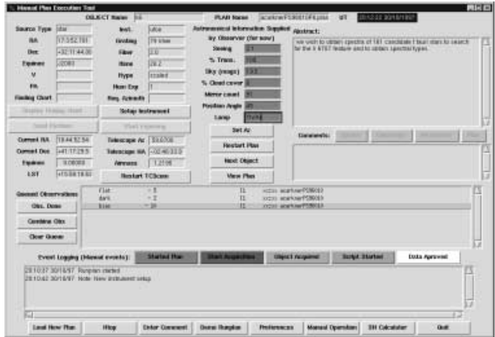
Figure 1. The plan execution tool reads in plan files and coordinates the observations with the other subsystems.
