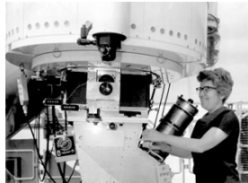
Vera Rubin, with DTM image tube spectrograph attached to the Kitt Peak 84-inch telescope, 1970.vv
