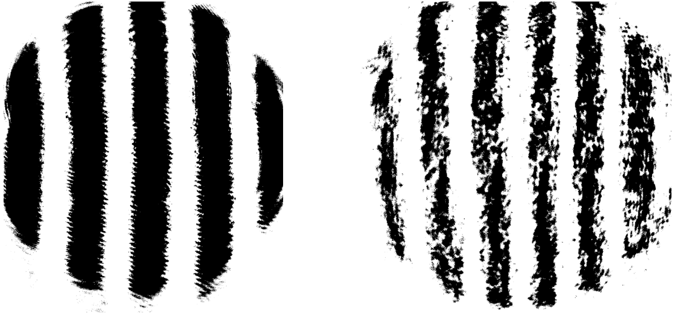
Figure 3. An interferogram in red light ( \lambda=632.8 nm, collimated beam 20 mm in diameter) of an unetched silicon disk surface (left) and an etched echelle grating in Littrow mode with fringes parallel to grooves (right).
