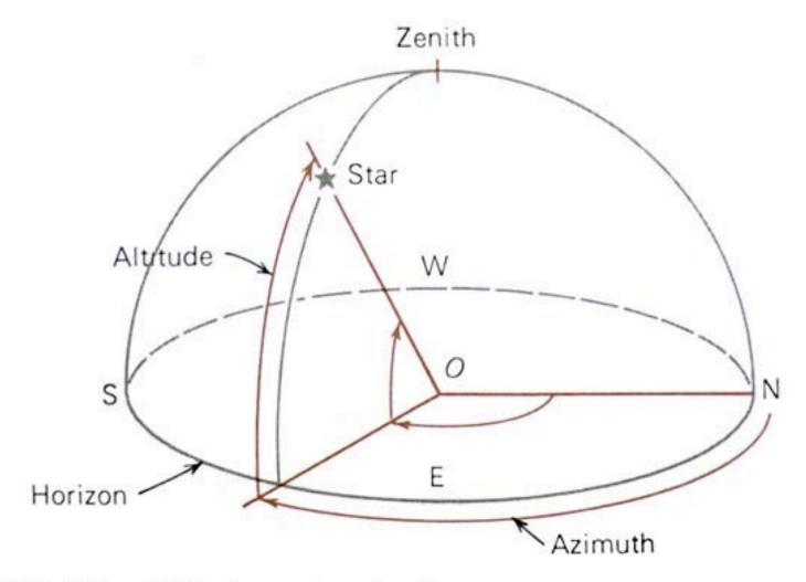
FIG. 5-3 Altitude and azimuth.
