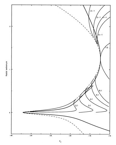
**Figure 7.** Characteristic curves showing the loci of the radial extrema of families of orbits which all close in one rotating frame; negative values are used for orbits which rotate in a sense counter to the frame. The thick line marks the circular orbits as a function of the Jacobi integral, and the dashed curve marks the ZVC which no orbit can cross. Each characteristic curve is marked with the *m:l* value for which the orbits close.
