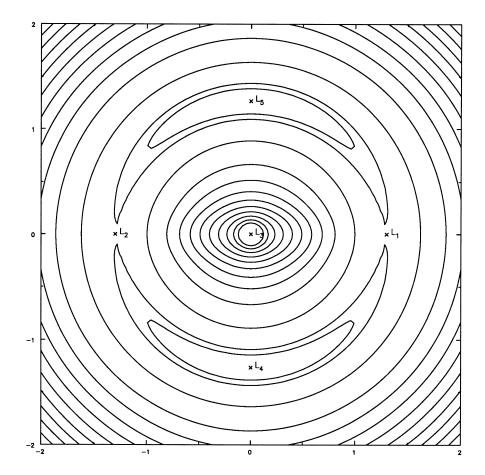
Figure 10. Contours of the effective potential in our barred model and the locations of the five Lagrange points. The  $L_3$  point at the centre is a minimum, the points marked  $L_4$  and  $L_5$  are equal absolute maxima and those marked  $L_1$  and  $L_2$  are saddle points. Well beyond this ring of Lagrange points, the effective potential slopes away parabolically to infinity. The bar major axis is across the page.
