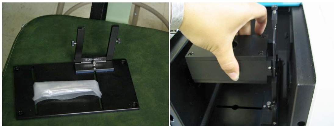
Figure 7: Base with screw bag (a) and box/tube being inserted into holder after base is screwed into the Cary (b).
