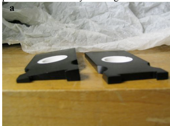
Figure 6: The 8 degree wedge on the left, and the 0 degree wedge on the right (a). The sides facing up in this picture would be the sides facing towards the rear for readings. Only use one wedge (either the 0 degree or the 8 degree) for each reading. You need to use the same wedge for your baseline as for you reading. Where the cord plugs in (b)
