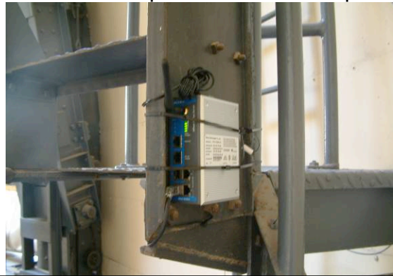
Picture 8: taken by Corby B. Bryan. MOXA UNIT on stairs above dome rotation point.
