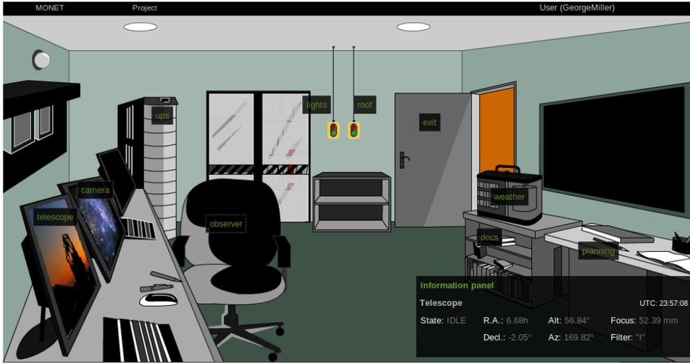
Fig. 8.—: The initial user interface for the MONET Telescope. Anyone has access to this window and can check the telescope’s position, focus, exposure time, etc. as well as the weather and roof.
