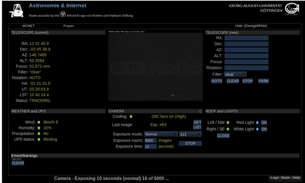
Fig. 9.—: The main telescope user interface where the telescope and camera are operated. The telescope’s position and status can be found in the left-most panel. The camera is controlled from the bottom panel. Exposure mode options are Normal, Dark and Bias. 1x1, 2x2 and 4x4 binning are available, but 2x2 binning should always be used for time series photometry. The telescope is operated from the right-most panel.
