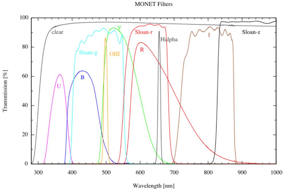
Fig. 7.—: Transmission curves for the available filters on the MONET telescope.
