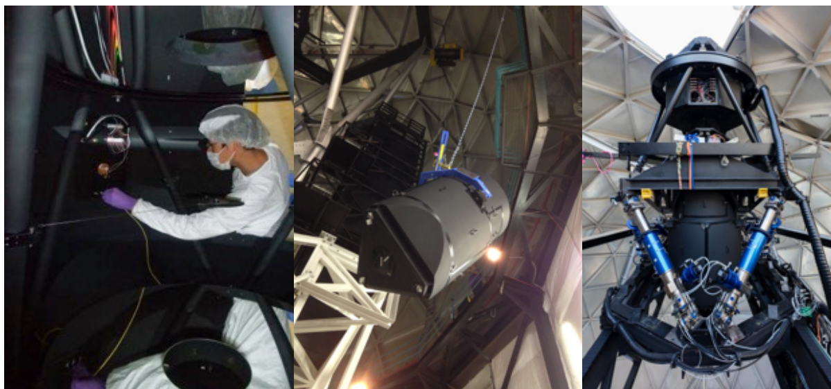
Figure 20 (Far left) Installing DMI fibers to the WFC instrument panel, (Left) WFC being lifted, (Right) WFC and the Prime Focus Instrument Package (PFIP) assembled on the HET tracker, (Far right) WFC + PFIP solid model.
