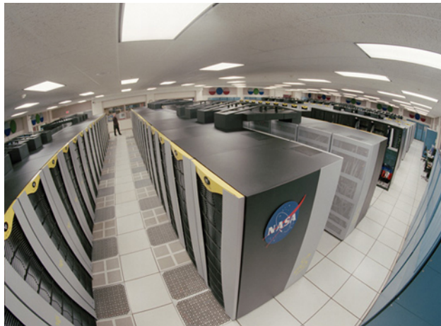
Figure 3.13. Modern Computing Power. These supercomputers at NASA's Ames Research Center are capable of tracking the motions of more than a million objects under their mutual gravitation. (credit: NASA Ames Research Center/Tom Trower)
