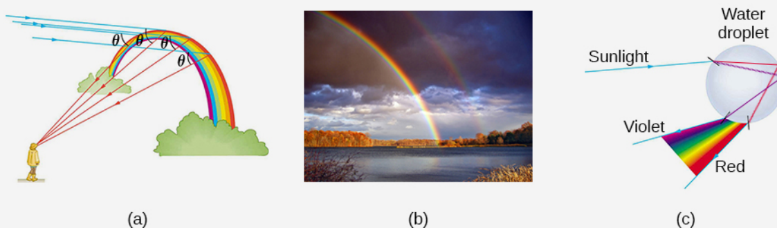
Figure 5.13. Rainbow Refraction. (a) This diagram shows how light from the Sun, which is located behind the observer, can be refracted by raindrops to produce (b) a rainbow. (c) Refraction separates white light into its component colors.
