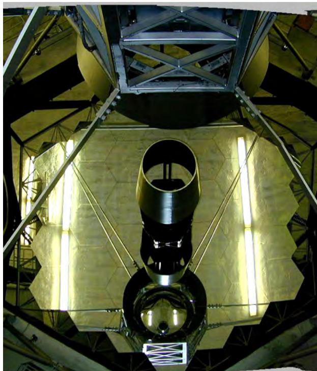
Figure 6.9. Thirty-Six Eyes Are Better Than One. The mirror of the 10-meter Keck telescope is composed of 36 hexagonal sections. (credit: NASA)
