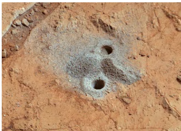
Figure 30.11. Mudstone. Shown are the first holes drilled by NASA's Curiosity Mars rover into a mudstone, with "fresh" drill-pilings around the holes. Notice the difference in color between the red ancient martian surface and the gray newly exposed rock powder that came from the drill holes. Each drill hole is about 0.6 inch (1.6 cm) in diameter. (credit: modification of work by NASA/JPL-Caltech/MSSS)
