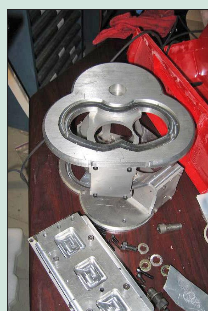
The binocular viewer housing ready for optics and final assembly
