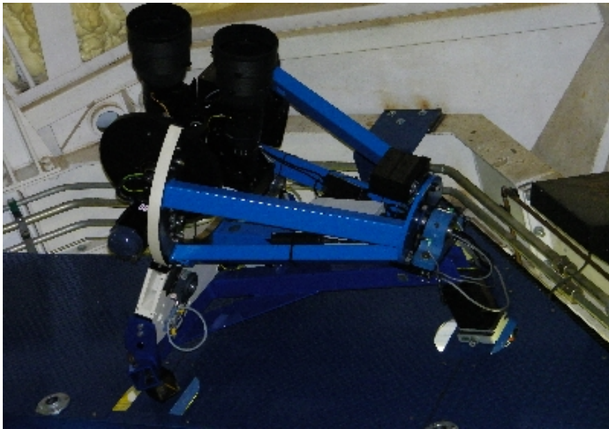
Four 14 cm telescopes. 4.5^\circ \times 4.5^\circ FOV
