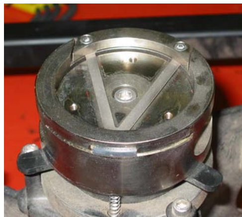
Figure 16. Flexure-mounted hub providing radial support of individual mirror segments.
