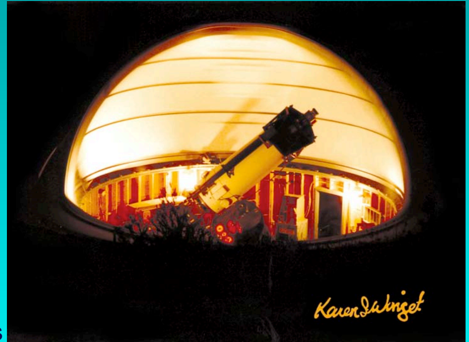
0.7m telescope with prime focus camera (22 nd magnitude in R in 15 minute exposure)
