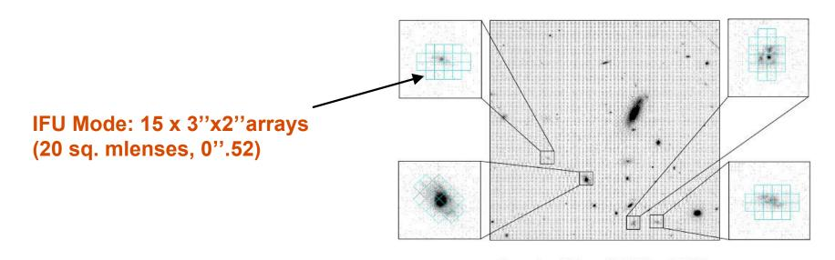
15 deployable IFUs over a 20 arcmin FoV with R<sub>effective</sub>= 13000
