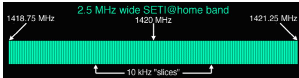
Figure 19.5 Concentrating a signal into a narrower bandpass makes it much easier for the signal to stand out against the background noise that exists at all frequencies.
