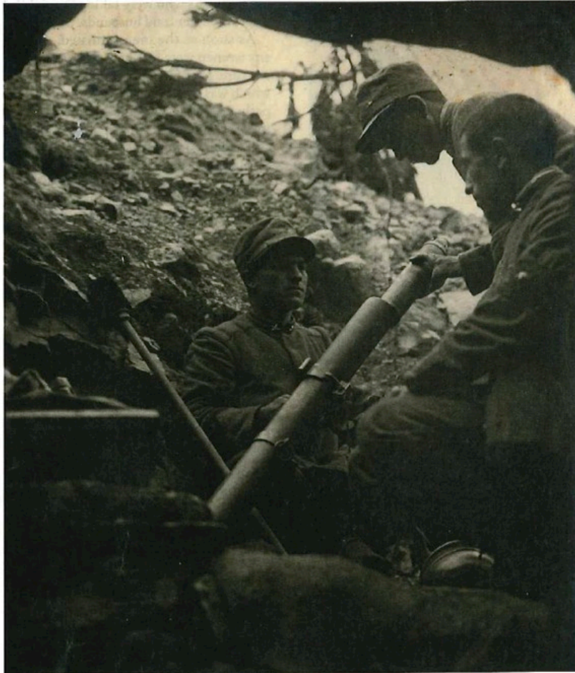
Soldiers load a Stokes mortar, invented in 1915 by engineer Wilfred Stokes for trench warfare.
