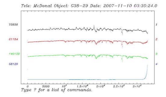
Figure 1: Example Wqed startup screen. The header tells you the telescope, object name and date and time of your first observation. The channel numbers, referring to the separate columns/stars in your input file, are found on the right. Use these numbers to select each channel/star. The number on left show the average number of counts in each channel.
